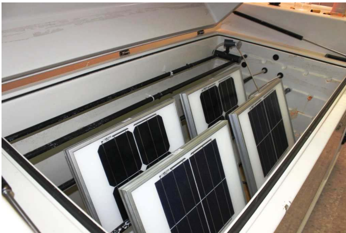
POSITIONING OF THE SAMPLES IN SALT SPRAY CHAMBER.
