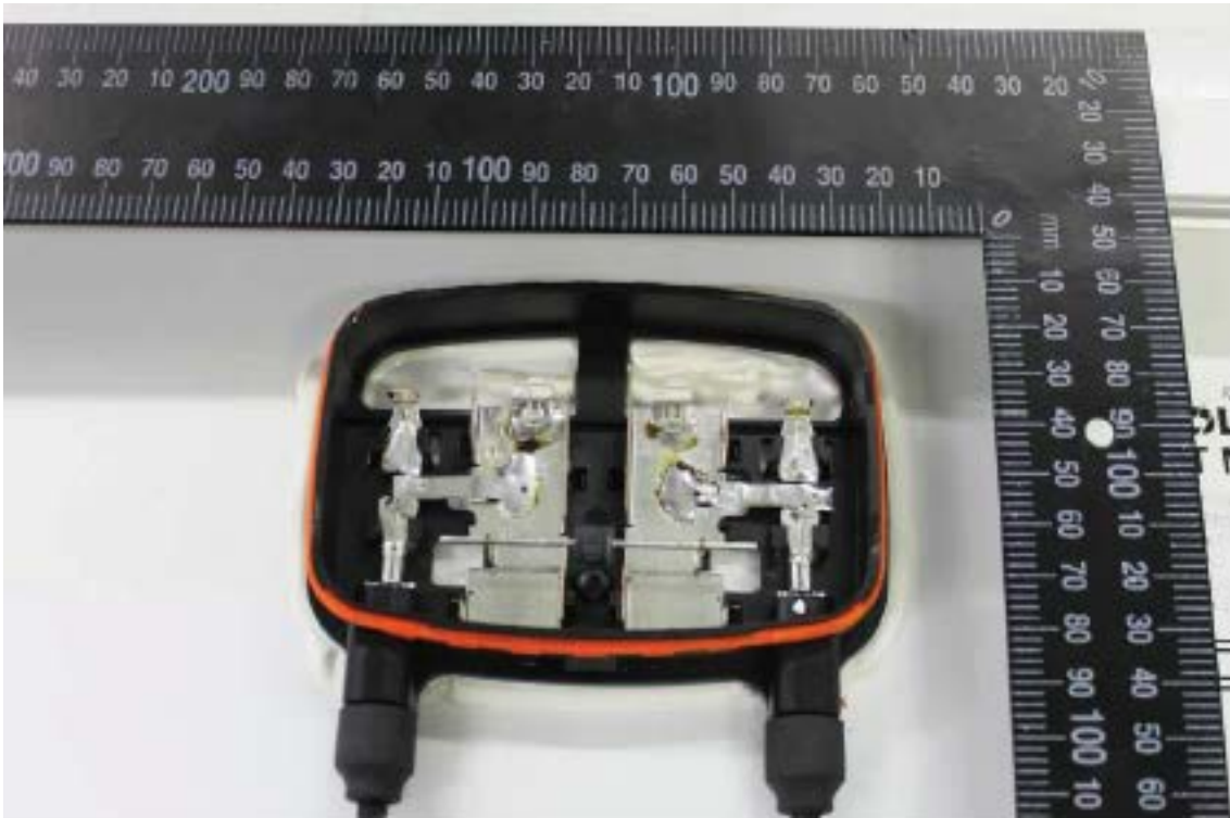
EXAMPLE OF THE JUNCTION BOX OPEN OF THE SAMPLE 41988/38.
