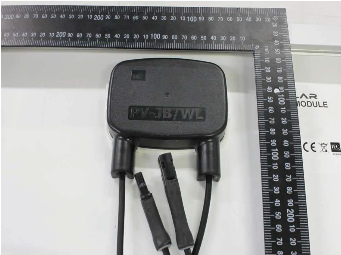
EXAMPLE OF THE JUNCTION BOX CLOSED AND CONNECTORS OF THE SAMPLE 41988/38.
